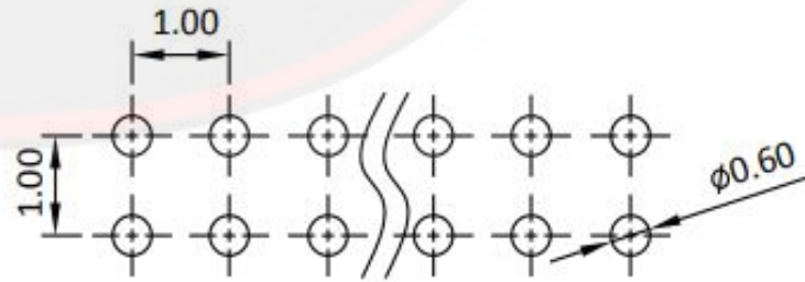
Recommended PCB Layout (PCB TOLERANCE ±0.05)
